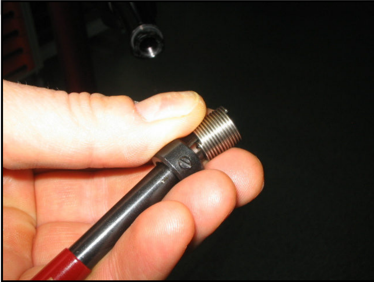
LEFTY SPINDLE HELI COIL REPLACEMENT
