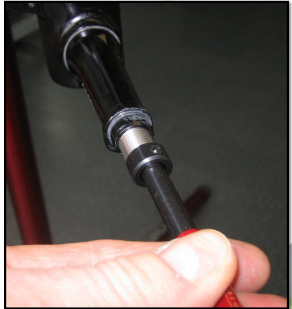
LEFTY SPINDLE HELI COIL REPLACEMENT
