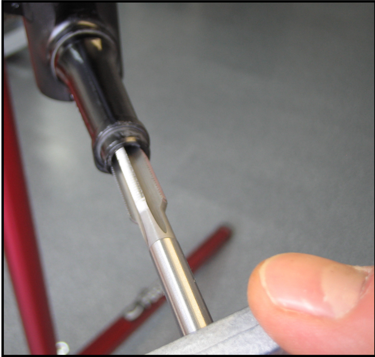
LEFTY SPINDLE HELI COIL REPLACEMENT
